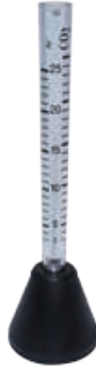
Gas flow rate meter
